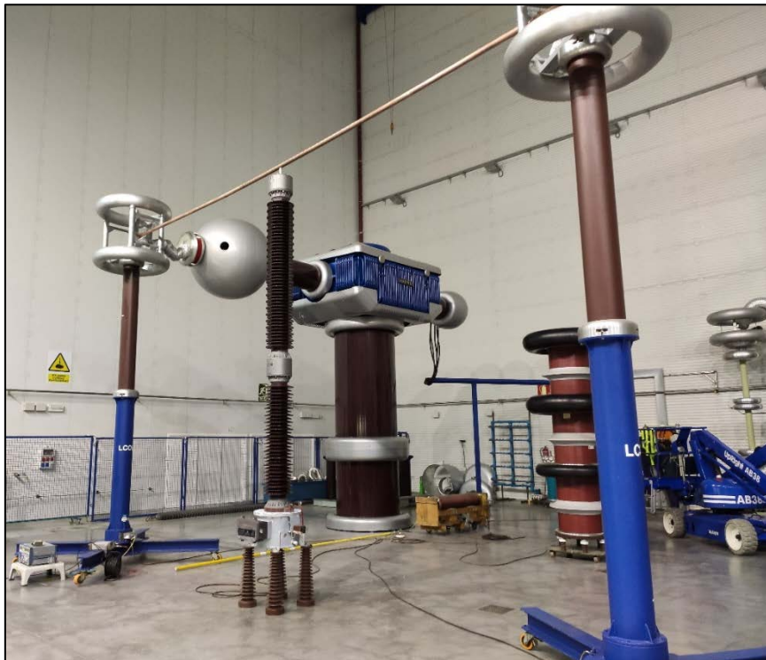
Power frequency generator up to 1 MV (50 Hz / 60 Hz)
