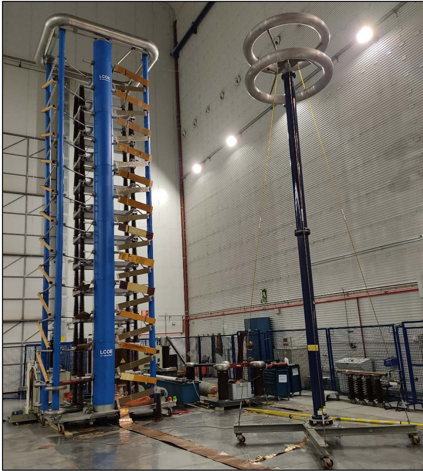
Impulse generator up to 2.4 MV
