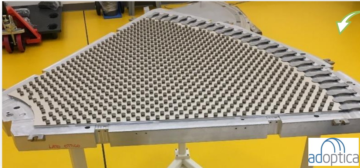
First finished Shell; back surface coated, equipped with glued magnets and lateral support (Oct'2020)
