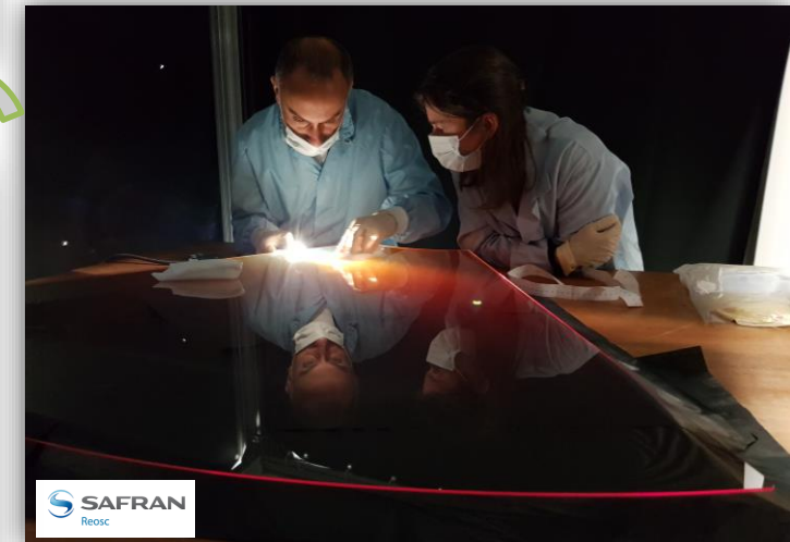
M4 Shells: Inspection after manufacturing by Safran Reosc (polishing/thinning/cutting)
